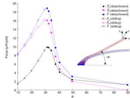
Figure 5. Analysis of the pull-off force of a single seta
