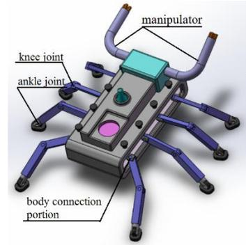
Figure 2 robot mechanism
