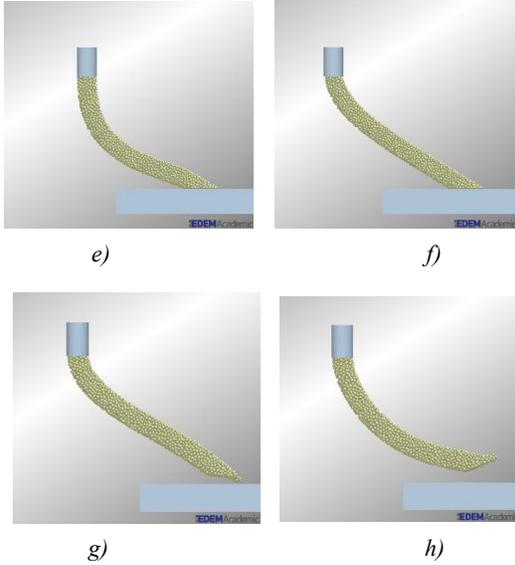
Figure 6. The simulation process of single fiber based on discrete element method
