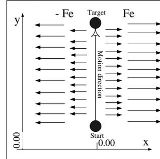
Figure 2: The unstable divergent force field (DF). The field force  $F_e$  is a function of position of slave object.
