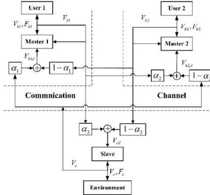
Figure 1: The system structure of dual-user shared control
