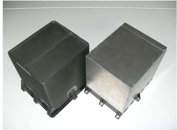
Figure 4: EMI CFRP- and reference-housing
