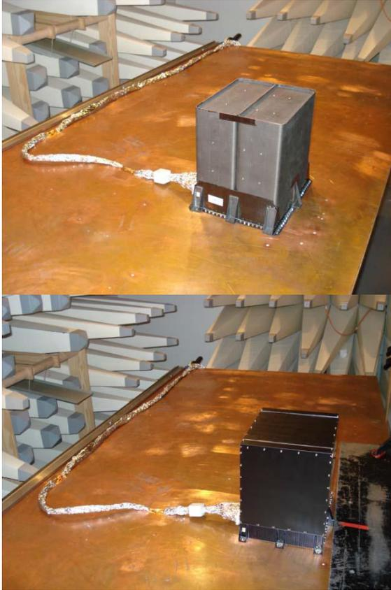
Figure 5: EMI CFRP housing (top) and reference housing (bottom) in the EMC test chamber
