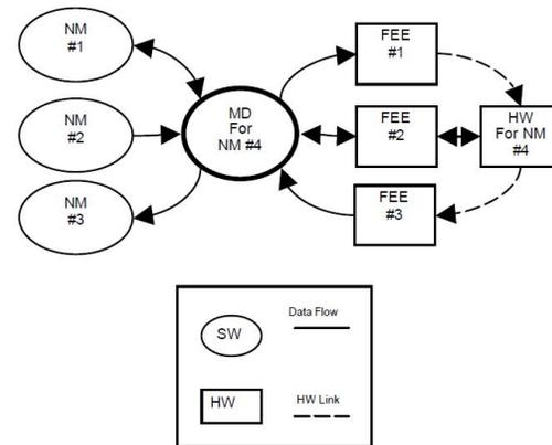
Figure 3: Hybrid model and architecture model composed of mathematical model and real hardware model
