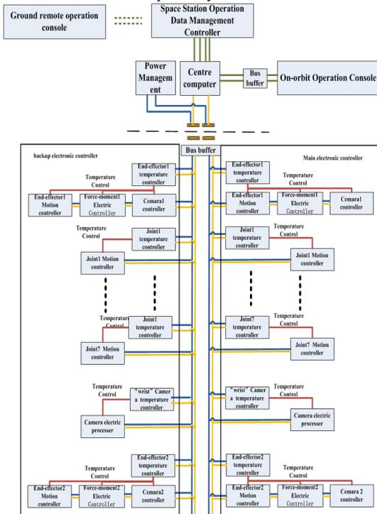
Fig.5 The distributed control system architecture of manipulator
