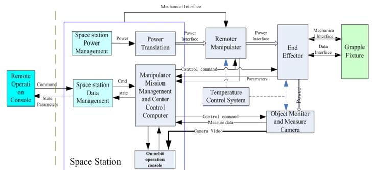
Fig.1 the system architecture of manipulator
