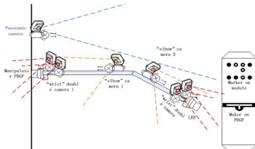
Fig.6 The configurations of artificial vision
