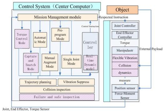
Fig.6 System architecture of centre computer
