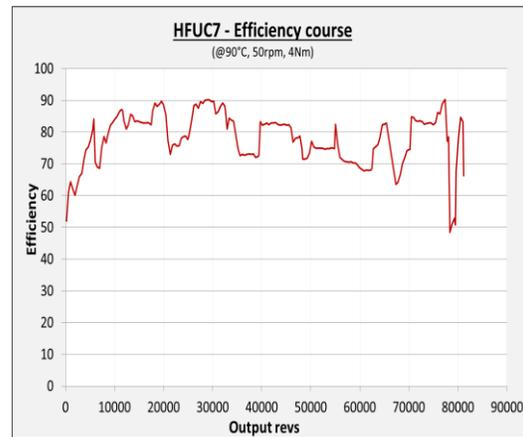
Figure16: MAC lubricated gearbox HFUC-7 during endurance testing at 90°C, 50rpm, 4 Nm
