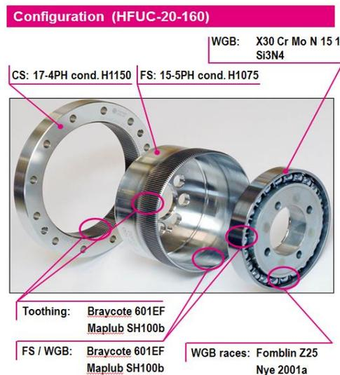
Figure 12: Configuration of gear material/lubrication
