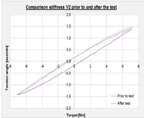
Figure 18: Stiffness prior to and after testing
