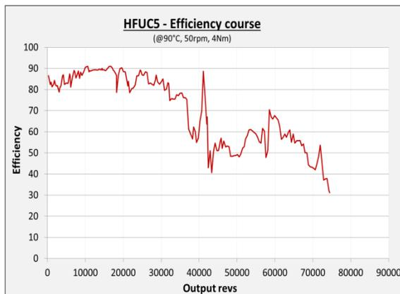
Figure15: Efficiency Course of PFPE lubricated gearbox HFUC-5 at 90°C, 50rpm, 4 Nm during endurance testing
