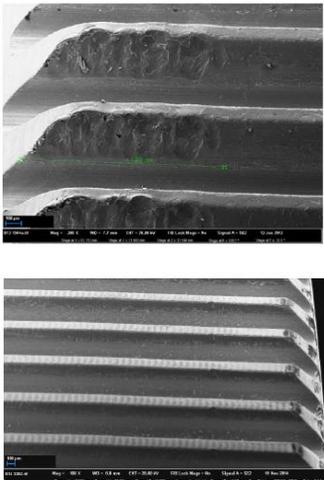
Figure 19: Upper SEM image of toothing after failure of endurance test in vacuum and lower SEM image of toothing after successful vacuum testing
