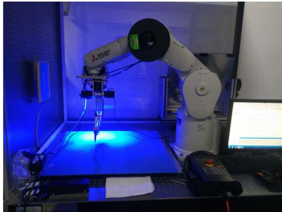
Fig.4 A robotic system with an end effector for 3D printing and a visual identification system
