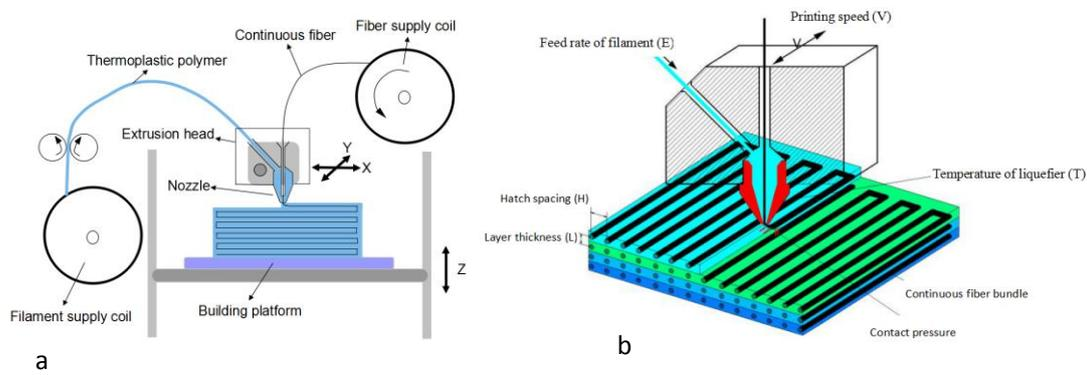
Fig. 1 Schematic of 3D printing equipment for CFRTPCs composites a), and scheme of the printing process b)
