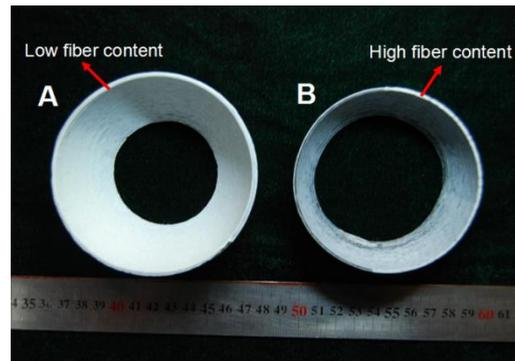
**Figure 6** Parts with different fiber contents: in the printing process, the feeding speed of thermoplastic material for part (A) is 1.5 times than the one of part (B), leading to the lower fiber content [3]
