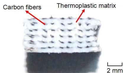
Figure 5 A consistent direction and an uniform distribution in composite parts [3]
