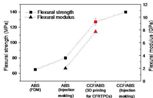
Fig.2 comparison of flexural strengths and modulus of ABS (FDM), ABS (injection molding), 10 wt% CCF/ABS (3D printing for CFRTPCs) and 10 wt% CCF/ABS (injection molding) (b)
