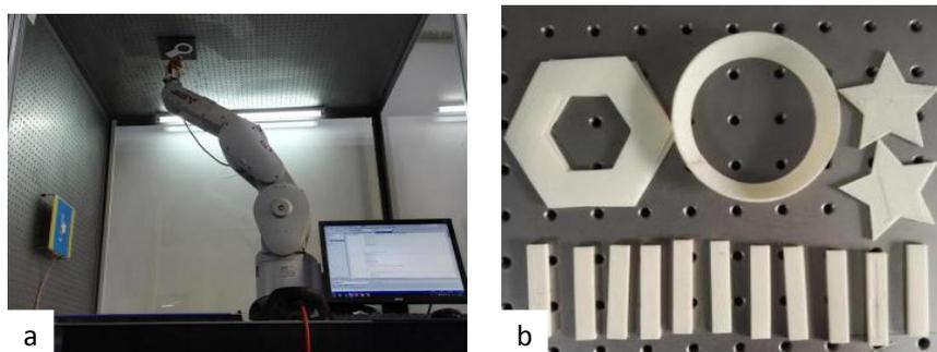
Fig.3 Robotic system for the 3D printing (a), and some samples fabricated by the robotic system (b)
