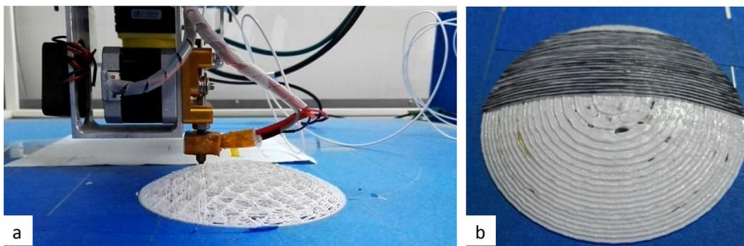
**Fig. 7** 3D printing process on a curved surface a) and deposited CFRTPCs on the curved surface b)
