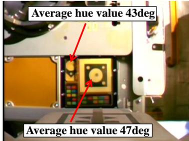
Figure 16: Measurement of hue value in ArrayMark's white area.
