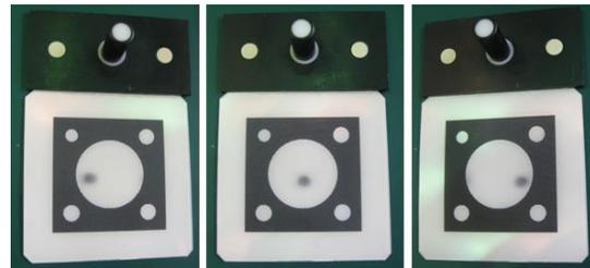
Figure 4: ArrayMark and 3D visual marker with rod. (three photos taken from different seeing-angles.)
