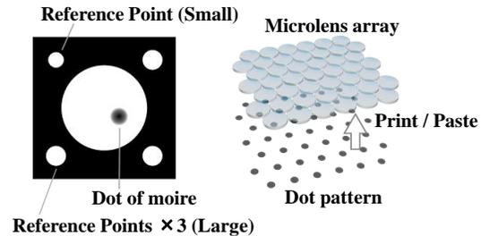
Figure 3: Design and structure of ArrayMark.
