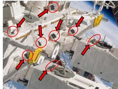
a) Visual marker attached on the ISS. ©NASA
