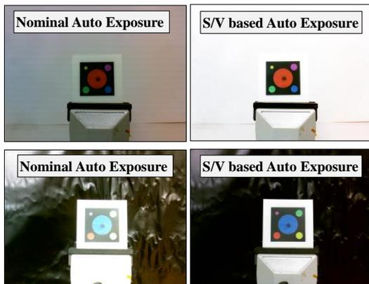
Figure 7: S/V-based adjustment of exposure as an image parameter. Unsuitable brightness of image is due to the nominal autoexposure function of the camera.
