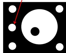
Figure 18: Suggested new ArrayMark design to improve position and attitude measurement accuracy in low-contrast images.
