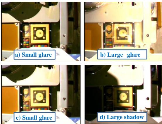
Figure 14: Example of glare or shadow on ArrayMark.
