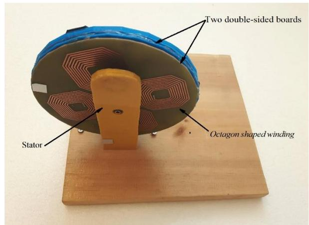
Figure 6: PCB rotor (octagon shaped winding)
