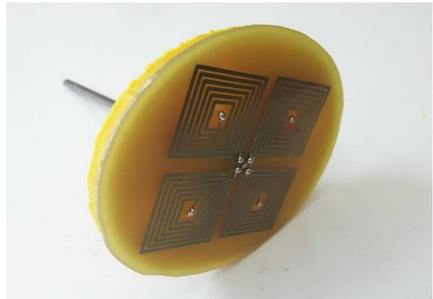
Figure 5: PCB rotor (Rectangularly shaped winding)
