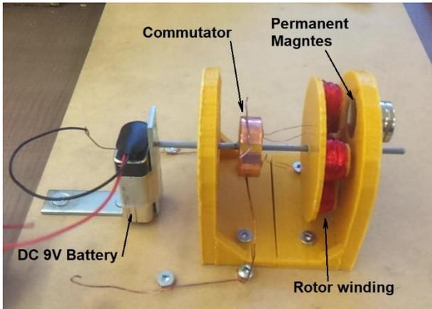
Figure 4: 3D printed DC brushed Pancake motor.
