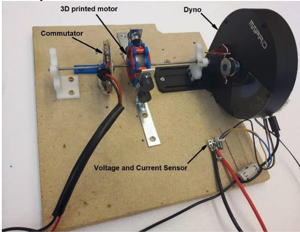
Figure 7: 3D printed DC motor connected to electric motor dyno
