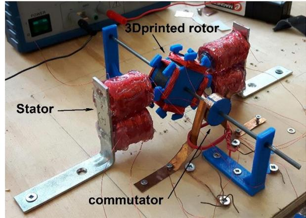
Figure 3: 3D printed Self-excited shunt DC motor.
