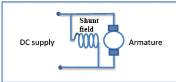
Figure 2: Self-excited shunt DC motor.
