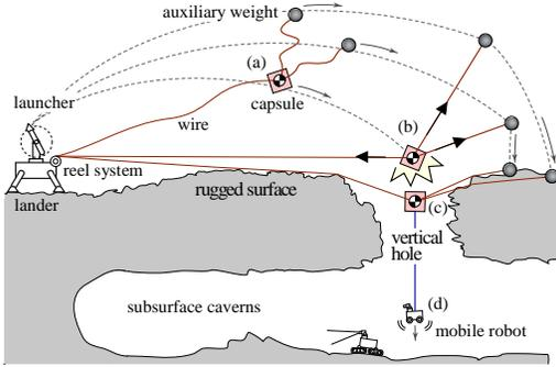
Figure 3: Scenario of delivering probe into the pit.
