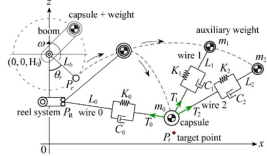
Figure 4: Model of launching system.
