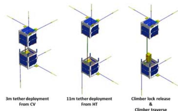
Figure 14. Tether deployment sequence.
