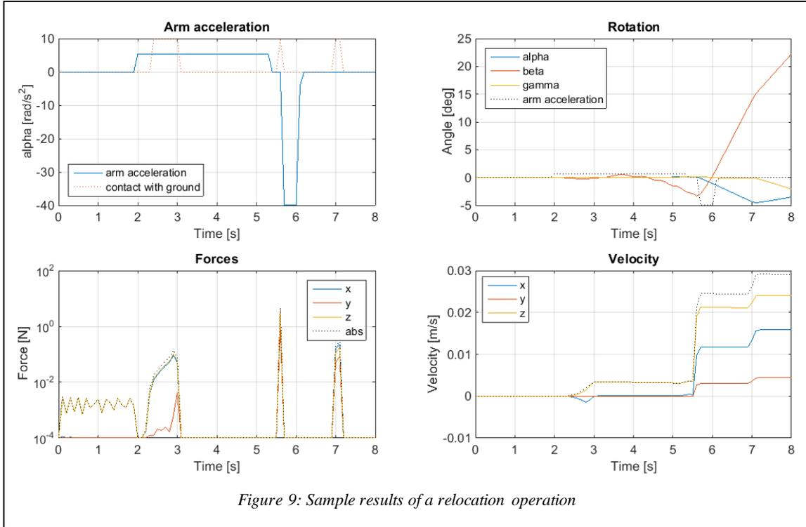
Figure 9: Sample results of a relocation operation
