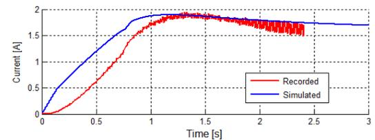
Figure 6: Prediction of the motor current
