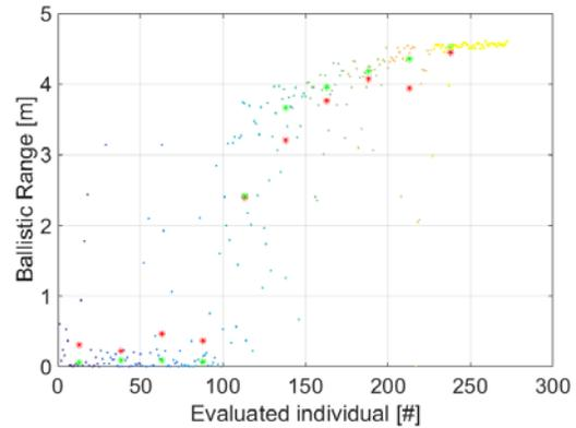
Figure 7: Successive evaluations of optimization criterion shows convergence under the assumptions of an ideal mobility
