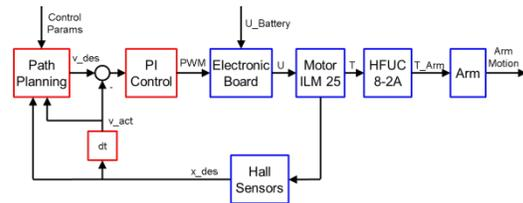
Figure 3: Block diagram of the mobility unit model
