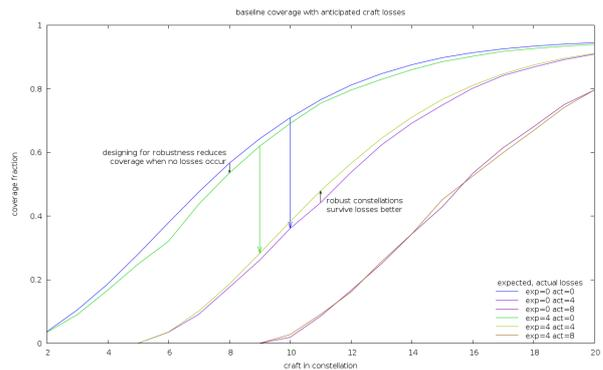
Figure 4: Explanatory plot of coverage metrics (out of 1.0) for solutions generated by using loss-sensitive optimization heuristic compared with the default heuristic. In situations with no realized losses, the loss-sensitive solution (green) fares worse than the naive solution (blue). However, when the predicted loss rate actually occurs, the loss-sensitive solution (yellow) dominates the naive solution (purple). At even higher loss rates, the solution difference becomes equivocal.
