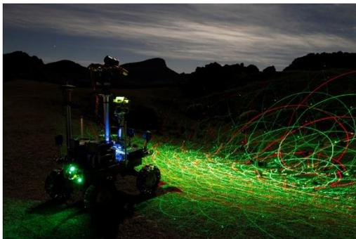
*Figure 3: GEPE with pattern projection system at work in Minas de San José.*
