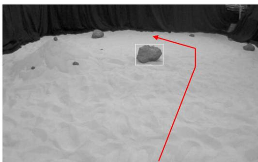
Fig. 5: Path planning result where three parameters are considered
