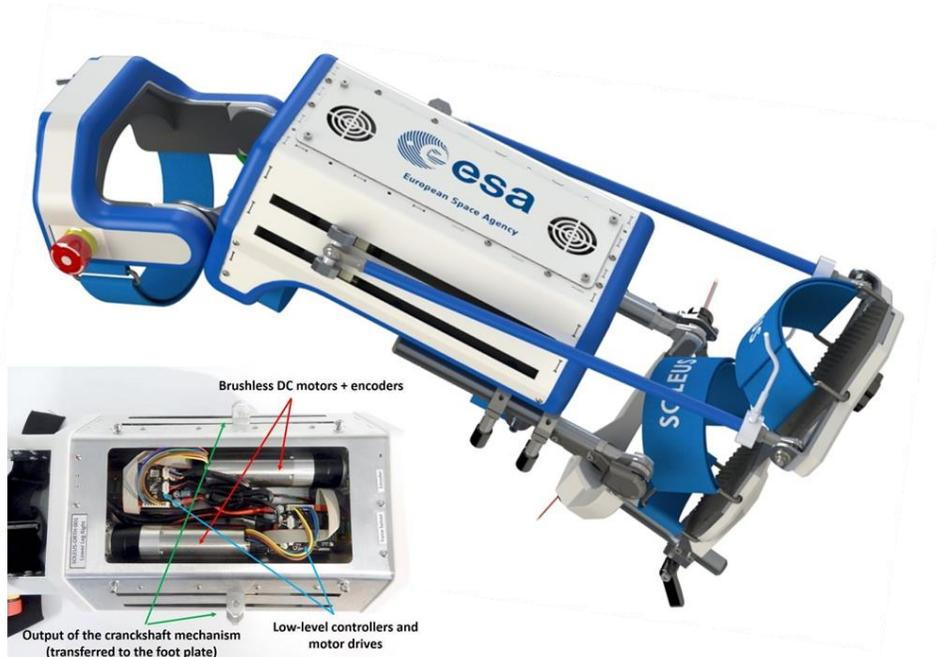
Figure 2: SOLEUS design and mechatronics highlights
