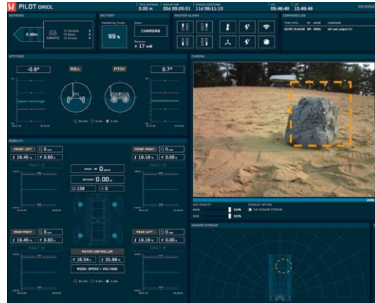
Figure 17: UI showing obstacle detection overlay on image and position on 2D map
