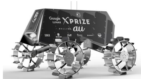
Figure 3: The “FM1” Sorato four-wheel rover
