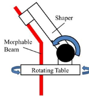
Figure 14: Beam shaper of Moving Beam Shaper
