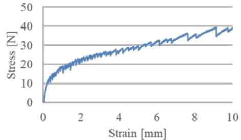
Figure 11: Stress-strain diagram (Stand tube (large)).
