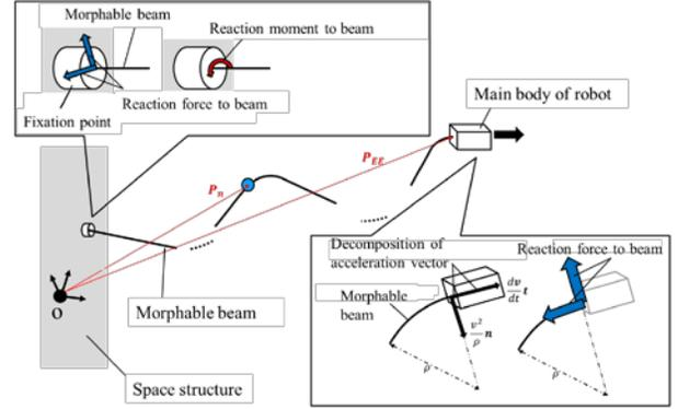
Figure 16: Reaction forces of the main body motion.
