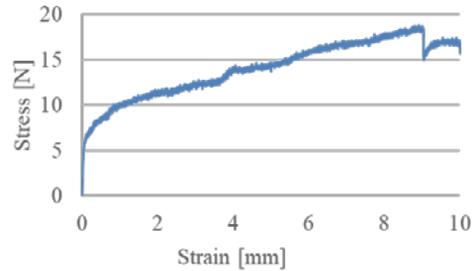
Figure 10: Stress-strain diagram (Stand tube (small)).
