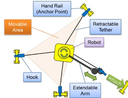
Figure 1: Tether-based locomotion
