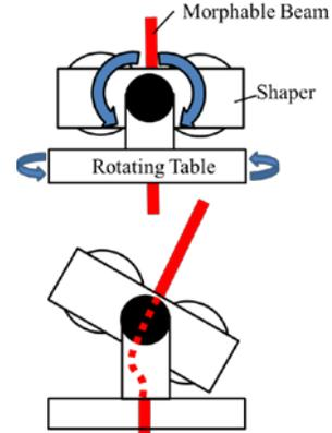
Figure 13: Beam shaper of MBD
