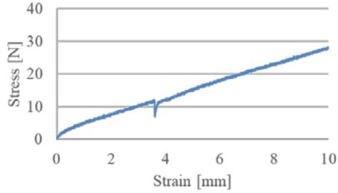
Figure 12: Stress-strain diagram (Casing carcass tube).
