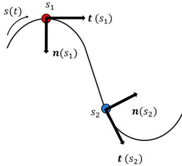
Figure 15: Motion of the mass point on the path of morphable beam
