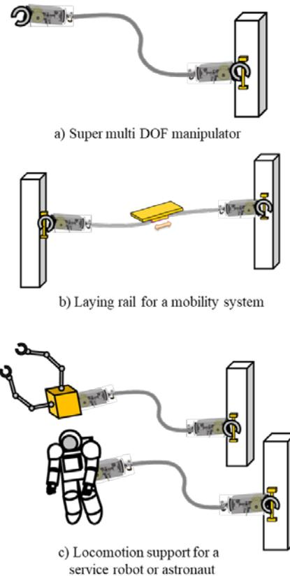
Figure 7: Application example of morphable-beam based Robot.
