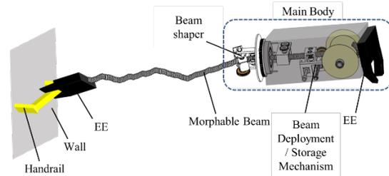
Figure 5: Basic concept of proposed morphable-beam based Robot.
