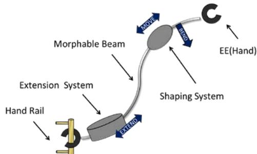
Figure 4: Moving Beam Shaper System [5]
