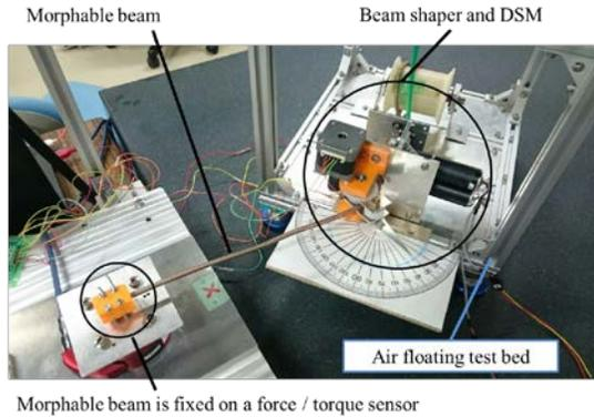
Figure 18: Experimental setup.
