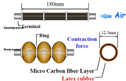
Figure 13: Structure and the driving principle of the straight fibers type soft actuator.
