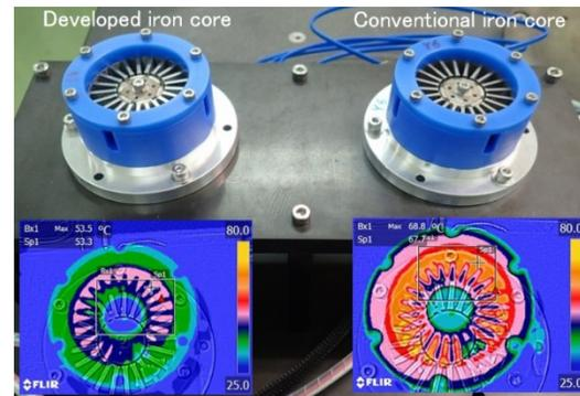
Figure 5. Heat characteristics of the commercialized motor of ShinMaywa (right) and a stator core replaced motor (left).
