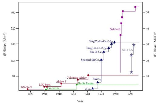
Figure 3. The development of permanent magnets in the 20th Century.  $BH_{max}$  has improved exponentially, doubling every 12 years [3].
