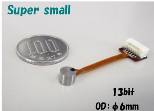
Figure 9: Super small resolver with thin flexible lead wire.
