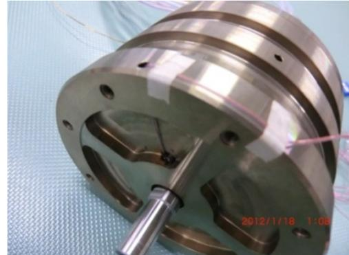
Figure 2. The DC brushless motor unit developed in JAXA.
