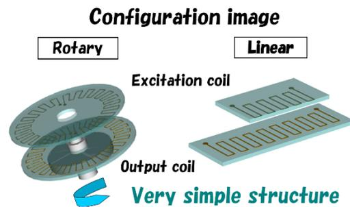
Figure 8: Configuration images of the resolvers.
