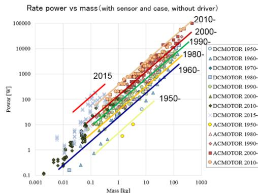
Figure 1. Power/mass ratio of the commercialized motors.
