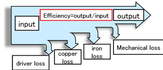
Figure 4: Classification of the motor loss.
