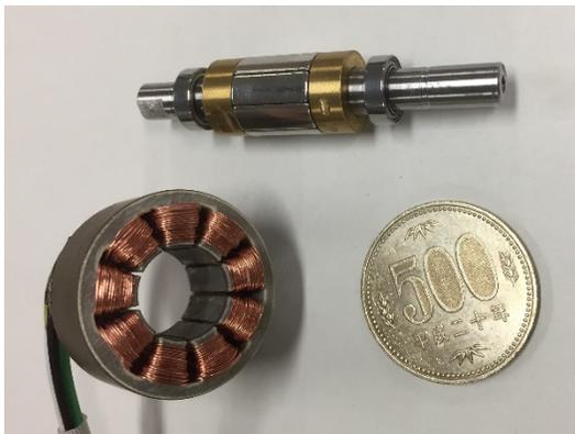
Figure 6. Rotor and the stator of the first prototype motor.
