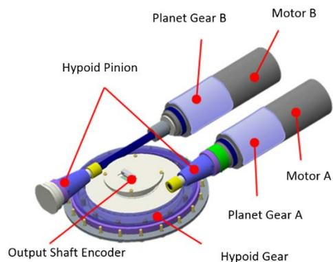
Figure 12: Basic structure of the power assist unit.
