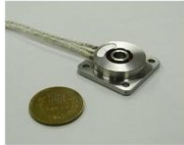
Figure 7. Modulated wave resolver developed in FY2012.
