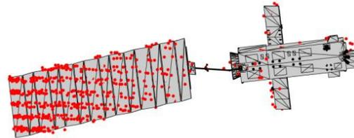
Figure 5. Matching result of JOP pose estimation algorithms between LIDAR scan and ENVISAT CAD model (bottom)
