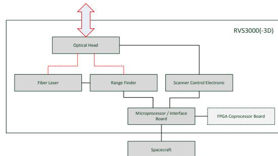
Figure 4. RVS3000 and RVS3000-3D simplified block diagram
