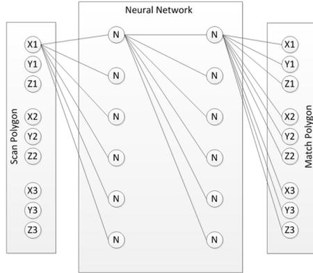
Figure 6. Calculation of a Match Polygon corresponding to a Scan Polygon sampled from a LIDAR Scan via a Feed-Forward Neural Network
