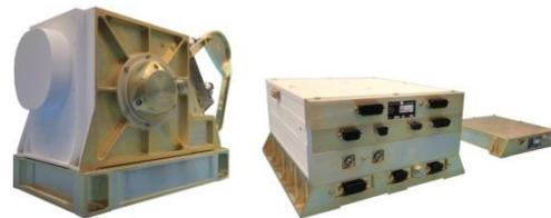
Figure 2. LIRIS-2 sensor components optical head, electronics box, and data recorder.
