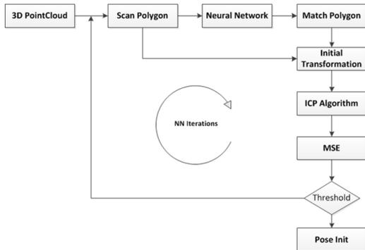
Figure 7. Pose Initialization Algorithm based on Poly-Matching via Neural Network
