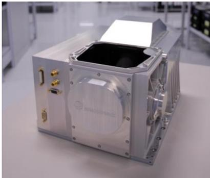
Figure 3. RVS3000 Engineering Model
