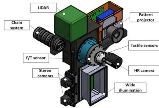
**Figure 14 – Housing of the orbital I3DS suite**
