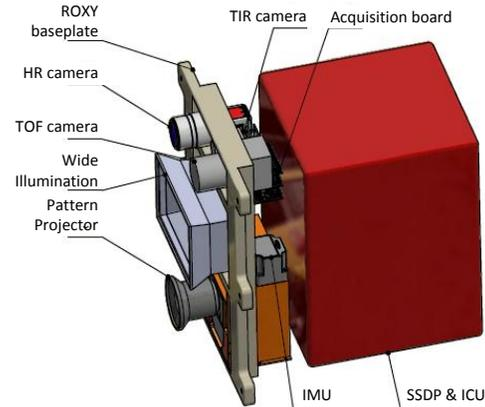
**Figure 15 – Housing of the planetary I3DS suite**
