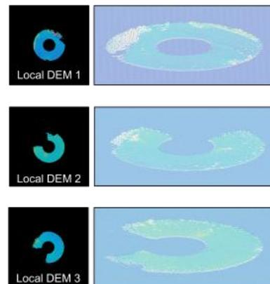
Figure 12 – Examples of consecutive DEM around the rover to build a global 3D map
