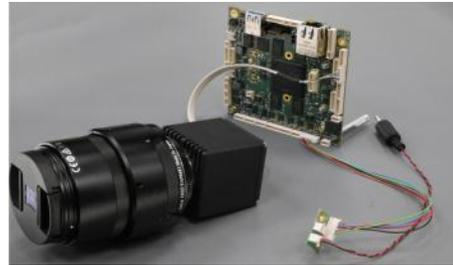
**Figure 7 - HR camera with electronic board**
