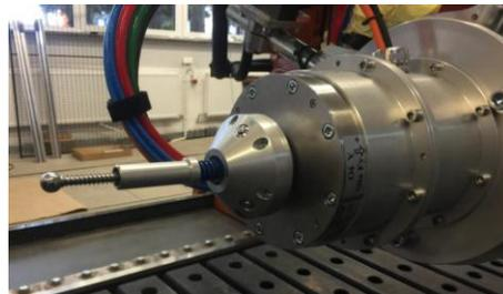
**Figure 9 - Contact unit (F/T & Tactile sensors)**
