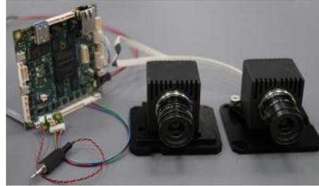
**Figure 6 - Stereo camera with electronic board**
