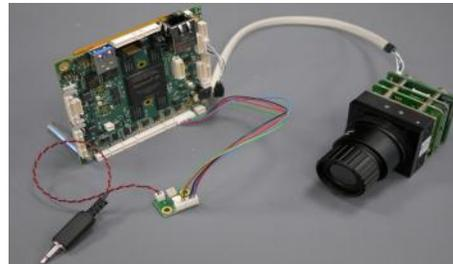
**Figure 8 - TIR camera with electronic board**
