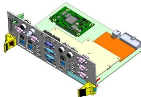
Figure 2 - ICU front panel and electronic cards
