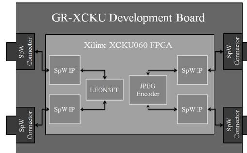
Figure 2: Processing Card 2 Architecture
