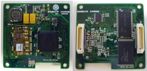
Figure 3: FPGA board
