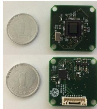
Figure 4: 3M pixel camera head board
