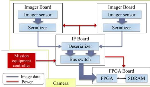
Figure 2: System diagram. FPGA: Field-programmable gate array; SDRAM: Synchronous dynamic random access memory.
