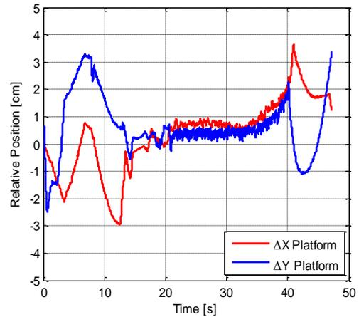
Figure 7: Relative positions of the platform with respect to the robot (zero gravity).
