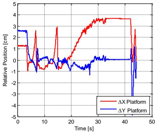
Figure 9: Relative positions of the platform with respect to the robot (artificial gravity).
