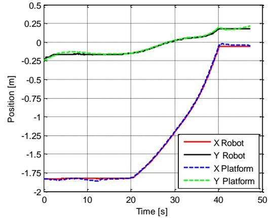
Figure 6: Positions of the platform and of the robot (zero gravity).
