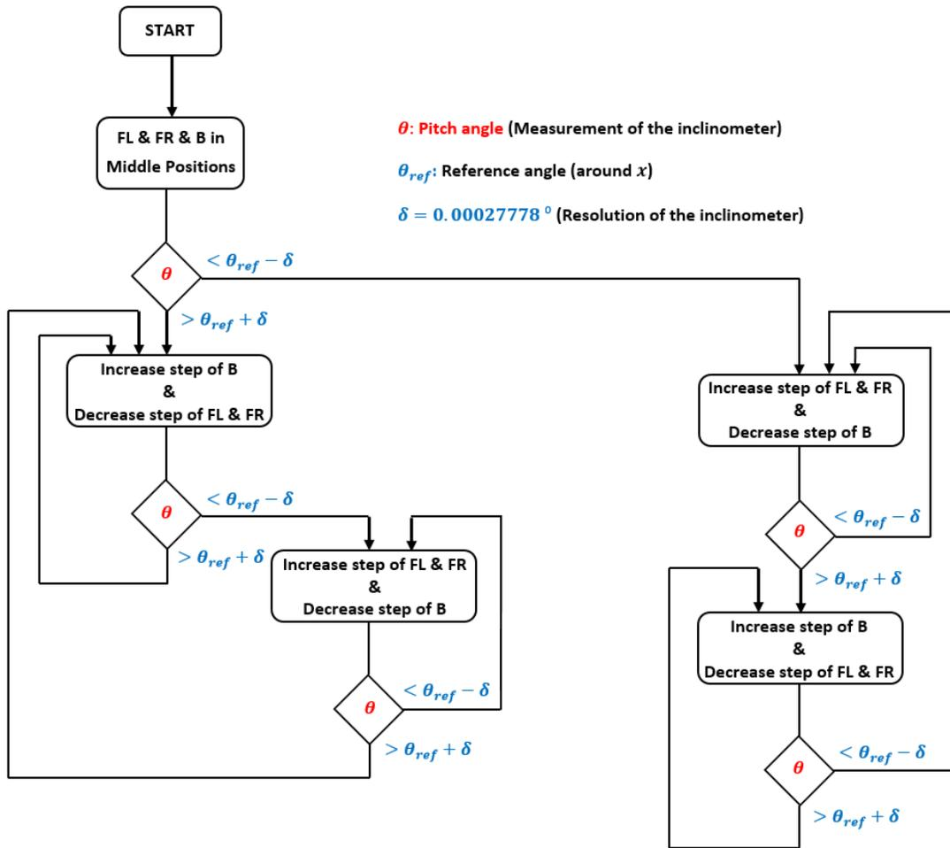
Figure 4: Flowchart of the control of the pitch angle,  $\theta$ .
