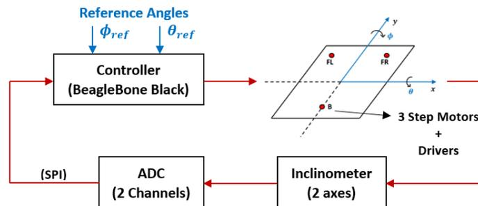
Figure 5: Block diagram of the controller.
