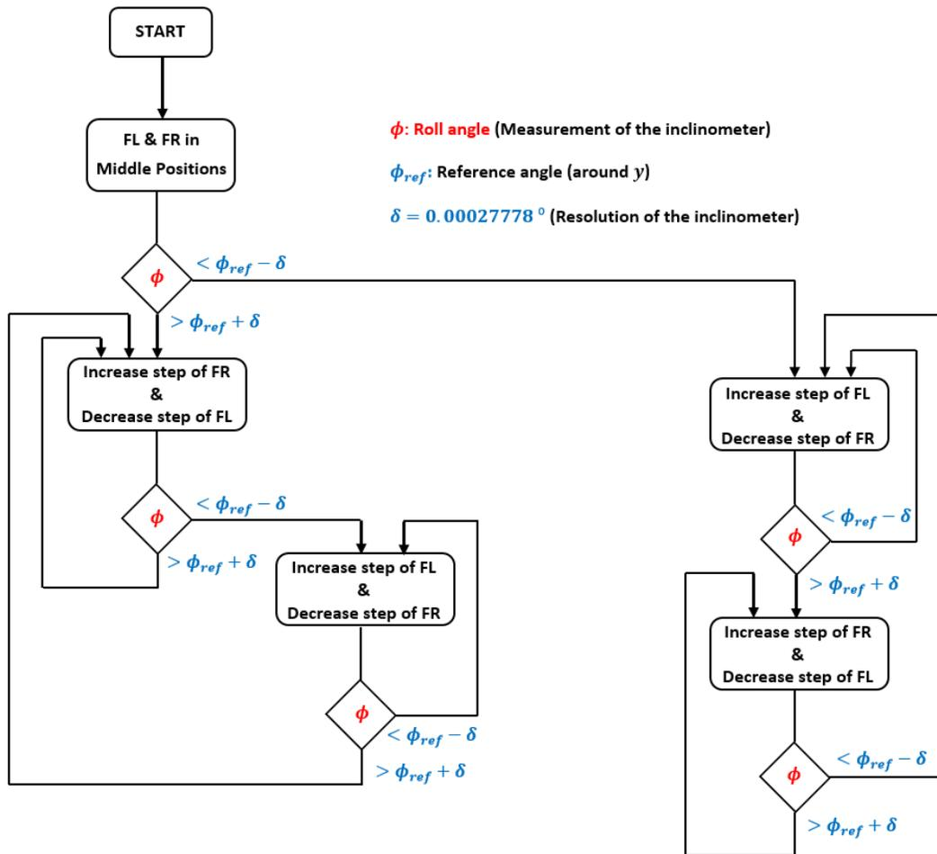
Figure 3: Flowchart of the control of the roll angle,  $\phi$ .
